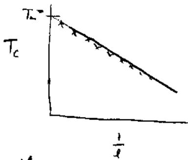
extrapolate the curve until it intersects the y-axis at  $T_m^0$
