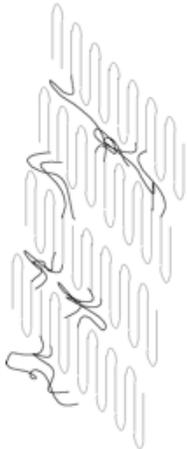
Stacks of chain folded lamellar crystals separated by amorphous regions. The degree of crystallinity is the lamellar thickness divided by the repeat distance,  $L$ .
