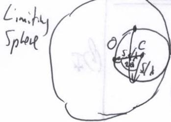
For the intersection of the Ewald sphere with a reciprocal lattice point rotating the lattice will trace out a circle on the surface of the Ewald sphere creating a Debye-Scherrer ring on the film which is part of the surface.
