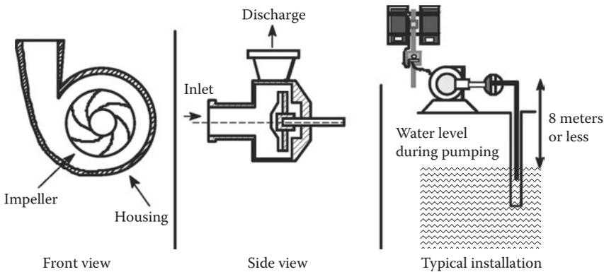
FIGURE 8.33 Diagram of a surface centrifugal pump.
