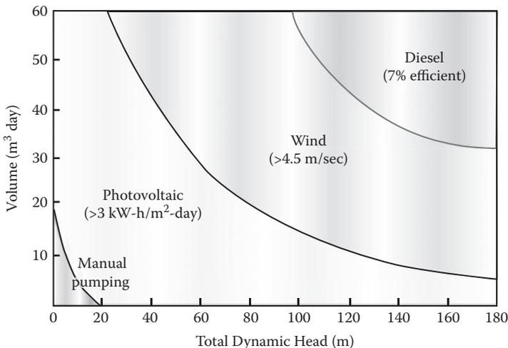
**FIGURE 8.28** Water-pumping technology selection based on hydraulic workload.
