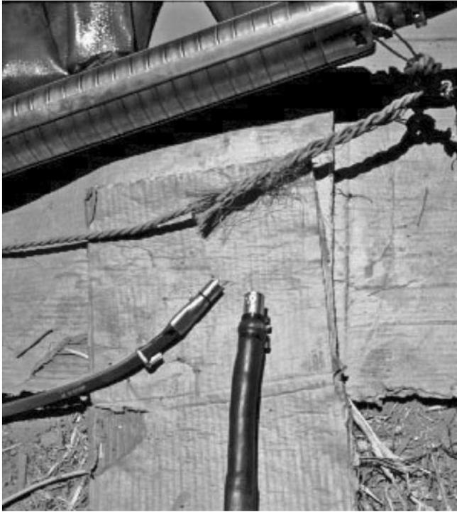
**FIGURE 8.43** PV pump damaged cable splice where conductors have worn through from hauling the pump up and down on the pump cable rather than the security rope (Roatan, Honduras).
