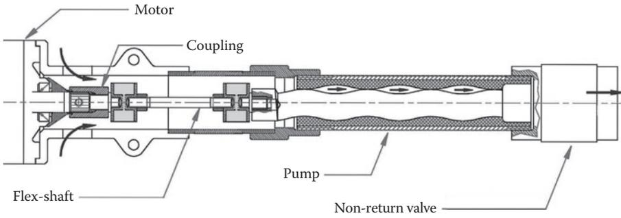
FIGURE 8.37 Diagram of a helical rotor pump.
