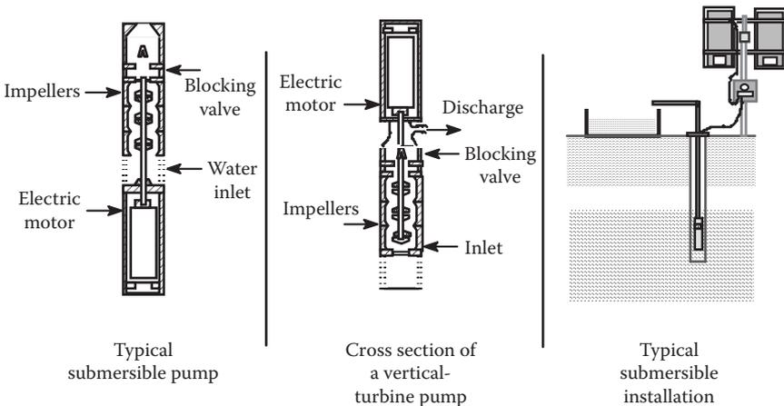
FIGURE 8.34 Diagram of a submersible centrifugal pump.
