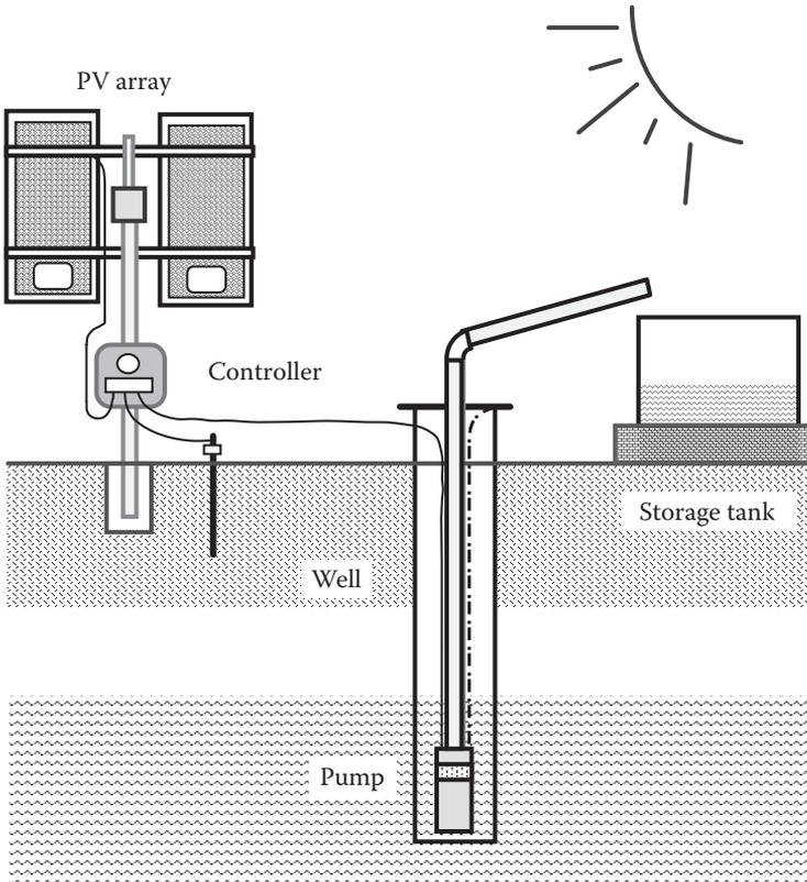
**FIGURE 8.31** A typical PV water pumping system.
