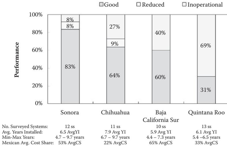
**FIGURE 8.45** Performance of Mexican PV water-pumping systems.
