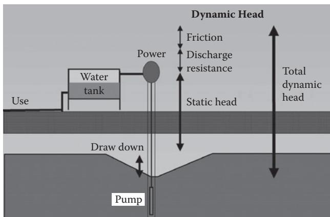
**FIGURE 8.30** Total dynamic head includes all components.
