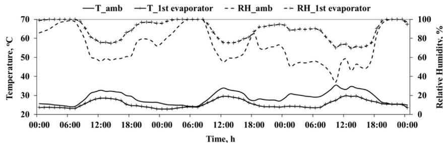
Fig. 7. Temperature and relative humidity changes across the first evaporator.
