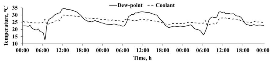
Fig. 11. Dew-point temperature of moist air and coolant temperature.
