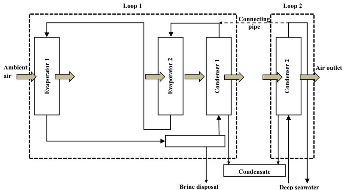
Fig. 3. Schematic of the suggested improvement on the design of SWGH in Oman [81].
