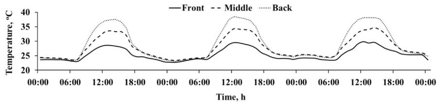
Fig. 9. Temperature gradient of air flowing through non-cultivated area of greenhouse.
