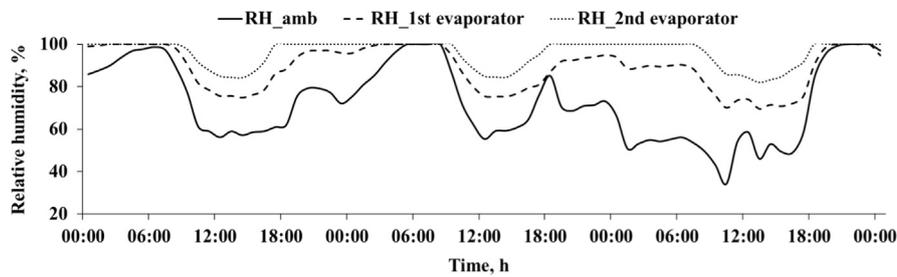
Fig. 10. Relative humidity of ambient air, after 1st evaporator and after 2nd evaporator.
