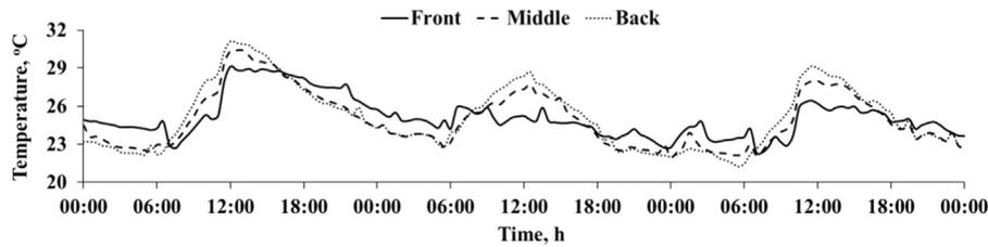
Fig. 8. Temperature gradient of air flowing through cultivated area of greenhouse.
