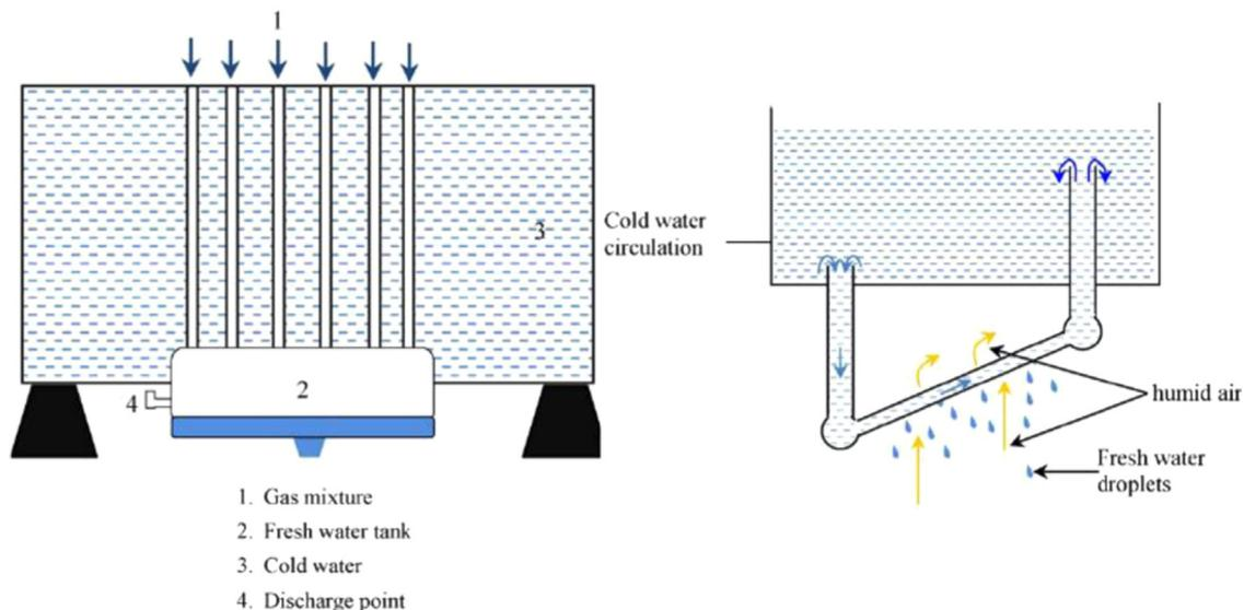
Fig. 4. Passive containment cooling systems; immersed-in-water condenser (left) and external passive condenser (right) [88].
