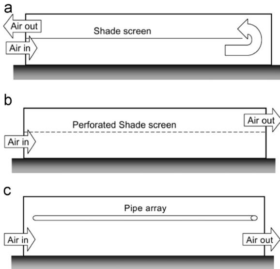
Fig. 2. Schematic of proposed airflow patterns; (a) elbow-shape air path, (b) air path through a perforated shade screen and (c) air path underneath a tube-array [61].
