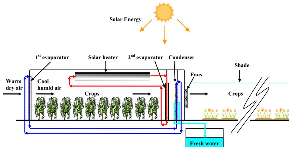
Fig. 1. Schematic of the SWGH in Oman.
