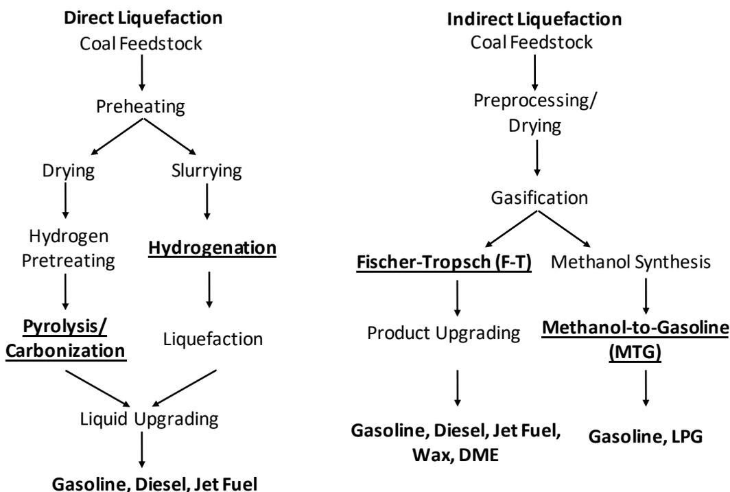
Each of the processes outlined in Exhibit 2-1 is chemically intensive compared to traditional oil refining [1], and have varying costs and potential profit margins. In terms of fundamental chemistry, the processes combine a carbon source with a H<sub>2</sub> source to form hydrocarbons of desired molecular weight range (synthetic crude oil or syncrude), which can be further refined into compounds that can reliably be mixed with traditional petroleum-based fuels.
