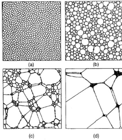
FIG. 4. Configurations of a foam consisting of 1000 bubbles with periodic boundary conditions as the volume is increased.  $V$  increases from (a) to (d): (a)  $V \ll V_{cr}$ ; (b)  $V \geq V_{cr}$ ; (c)  $V > V_{cr}$ ; (d)  $V \gg V_{cr}$ .
