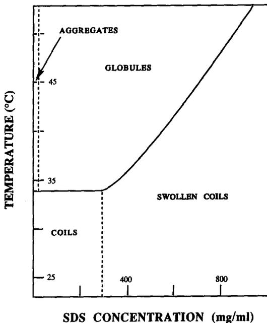
FIG. 20. Phase diagram of PNIPAAm and solution dodecyl sulfate (SDS) in water.
