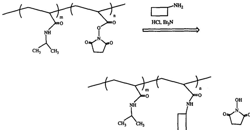
FIG. 3. NASI scheme for synthesizing functional PNIPAAm.
