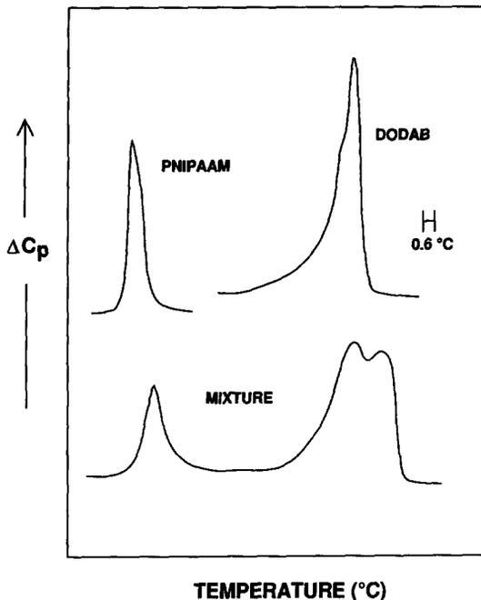
FIG. 18. DSC of PNIPAAm and DODAB solutions and their mixture. Heating rate: 15°C/hr.
