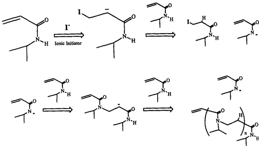
Fig. 2. Mechanism for hydrogen transfer polymerization.
