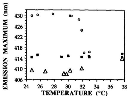
FIG. 10. Following the LCST of PNIPAAm ( $0.4 \text{ mg/ml}$ ) polymers with C12NS as a probe. PNIPAAm ( $\circ$ ), PNIPAAm-HDAAM  $0.4\%$  ( $\blacksquare$ ), PNIPAAm-HDAAM  $1.1\%$  ( $\triangle$ ).
