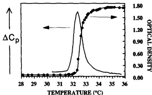
FIG. 4. Cloud point and DSC measurements of the LCST of PNIPAAM chains (0.4 mg/ml).
