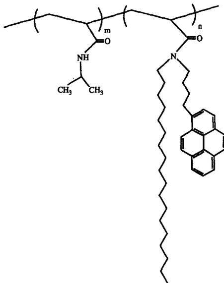
FIG. 7. Fluorescent, hydrophobically-modified PNIPAAm.
