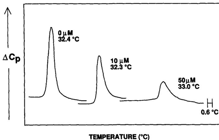
FIG. 19. DSC of the effects of SDDSS on the LCST of PNIPAAm. Heating rate: 15 $^{\circ}\text{C}/\text{hr}$ .
