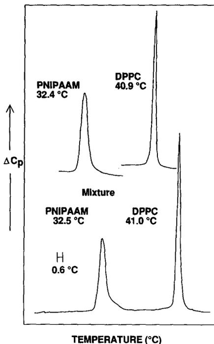
FIG. 17. DSC of PNIPAAm and DPPC solutions and their mixture. Heating rate:  $15^{\circ}\text{C}/\text{hr}$ .
