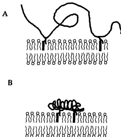
FIG. 16. "Molecular Accordion" effect for PNIPAAM in lipid bilayers.
