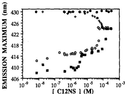
FIG. 8. Interactions of PNIPAAm and copolymers with C12NS. Water alone ( $\bullet$ ), PNIPAAm (+), PNIPAAm-HDAAM 0.4% (O), PNIPAAm-HDAAM 1.1% ( $\blacksquare$ ) at 0.4 mg/ml of each polymer; measurements at 24.5°C.
