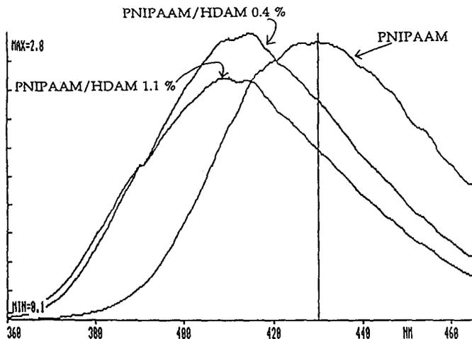
FIG. 9. Spectra for PNIPAAm and copolymers with added C12NS.
