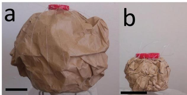
Fig. 2 (a) Experimental setup consisting of a net of wires distributed uniformly around a loosely crumpled sheet, which pass through a hole in the platform on which the crumpled sheet is placed. (b) By hanging weights at the bottom of the net one achieves higher degree of quasi-isotropic compaction. The scales are 2 cm.
