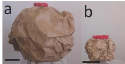
Fig. 2 (a) Experimental setup consisting of a net of wires distributed uniformly around a loosely crumpled sheet, which pass through a hole in the platform on which the crumpled sheet is placed. (b) By hanging weights at the bottom of the net one achieves higher degree of quasi-isotropic compaction. The scales are 2 cm.
