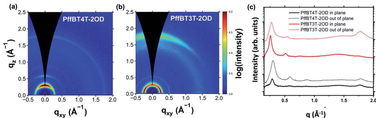
Fig. 5 2D GIWAXS images of polymer thin films; (a) PffBT4T-2OD and (b) PffBT3T-2OD. (c) Integrated scattering intensity of GIWAXS measurements shown in (a) and (b).
