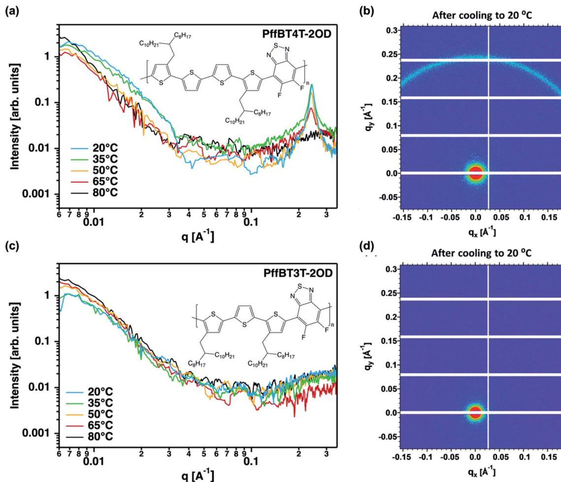
Fig. 1 Solution small-angle X-ray scattering (SAXS) 1D profiles for (a) PffBT4T-2OD and (c) PffBT3T-2OD in a solvent mixture of oDCB : CB [1 : 1] at different temperatures (20 to 80 °C). At  $q > 0.02 \text{ \AA}^{-1}$  intensity values were smoothed with 10 point moving average to reduce the noise. 2D plots taken at 20 °C are shown for PffBT4T-2OD and PffBT3T-2OD in (b) and (d) respectively.
