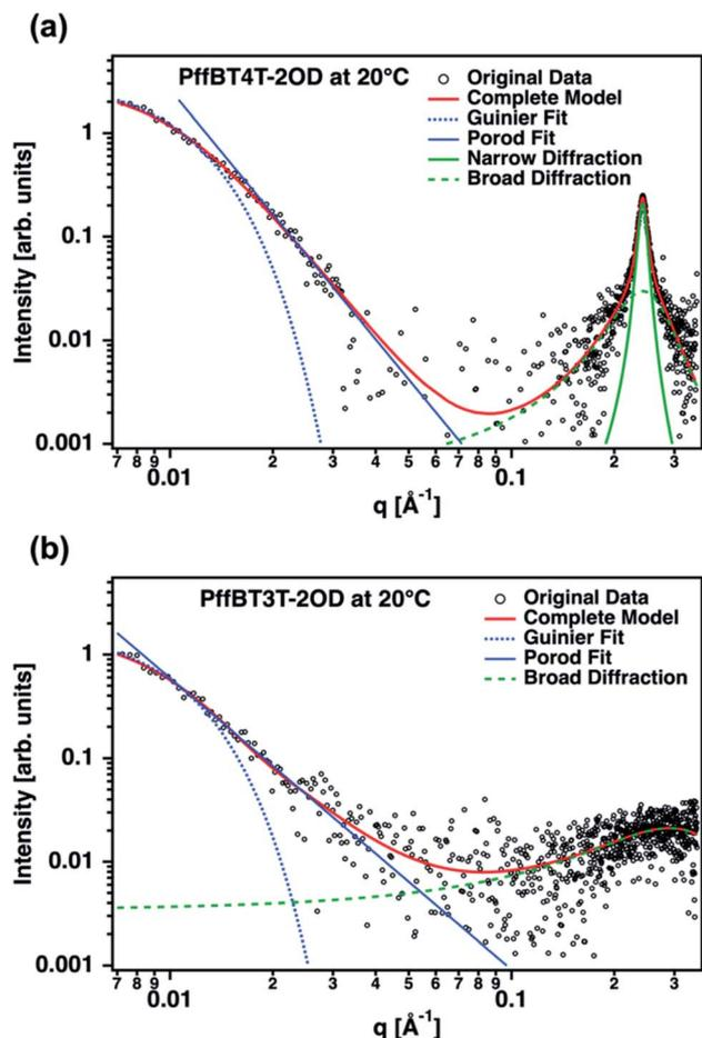
Fig. 2 Solution small-angle X-ray scattering (SAXS) profiles and their fits for PffBT4T-2OD and PffBT3T-2OD in a solvent mixture of oDCB : CB [1 : 1] at 20 °C in (a) and (b), respectively. The low  $q$  range in (a) and (b) was fitted with a unified fit model that relies on combination of Porod's and Guinier's law. The high  $q$  range in (a) was fitted using Lorentzian curves.
