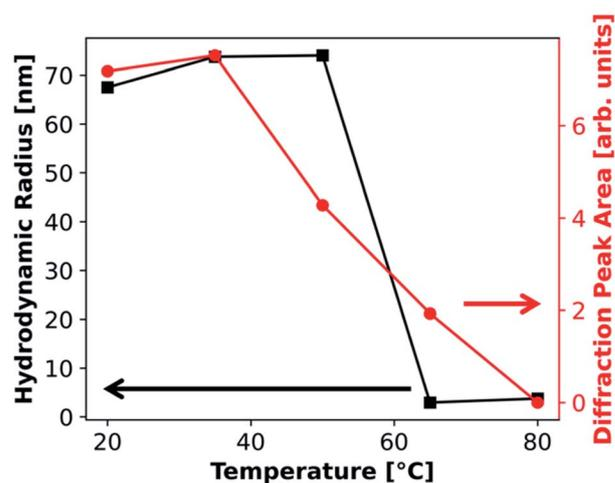
Fig. 3 Hydrodynamic radius reported from DLS measurements and narrow diffraction peak area reported from solution SAXS measurements as a function of temperature for PffBT4T-2OD. Similar transitions around 50 °C from both measurements demonstrate temperature dependent aggregation.
