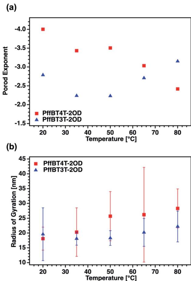
Fig. 4 Porod exponents (a) and radius of gyration values (b) extracted from model fits for PffBT4T-2OD and PffBT3T-2OD SAXS profiles. We were unable to calculate error bars for the Porod exponent due to high noise level in the data.
