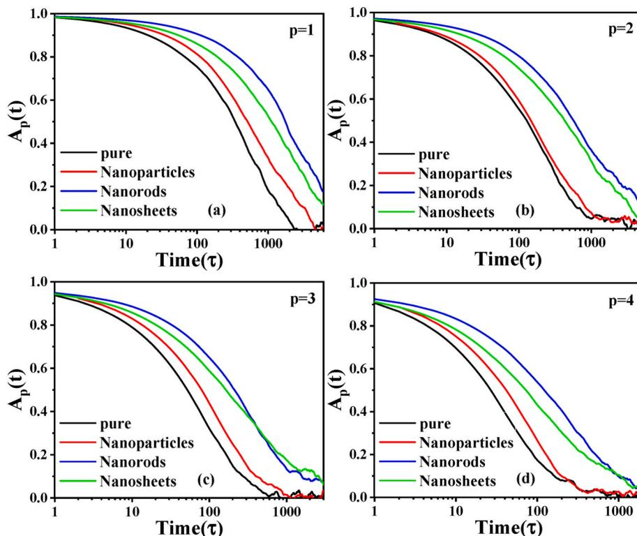
Fig. 5. Plots of  $A_p(t)$  functions for the four modes (a)  $p = 1$  (b)  $p = 2$  (c)  $p = 3$  (d)  $p = 4$  of the PNCs filled with different shape fillers at  $\phi = 5\%$ .
