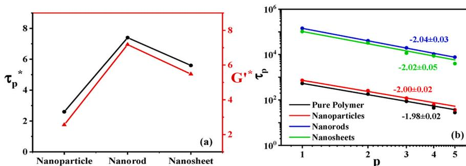
**Fig. 6.** (a) Ratio of relaxation time  $\tau_p$  and energy storage modulus  $G'$  of PNCs filled with different shape fillers to that of pure polymer at  $\varphi = 5\%$ , where  $\tau_p^* = \tau_p(i)/\tau_p(\text{polymer})$ ,  $G^* = G'(i)/G'(\text{polymer})$ ,  $i$  means nanoparticles, nanorods, nanosheets. (b) Fitting relaxation time of PNCs filled with different shape fillers at  $\varphi = 10\%$ .
