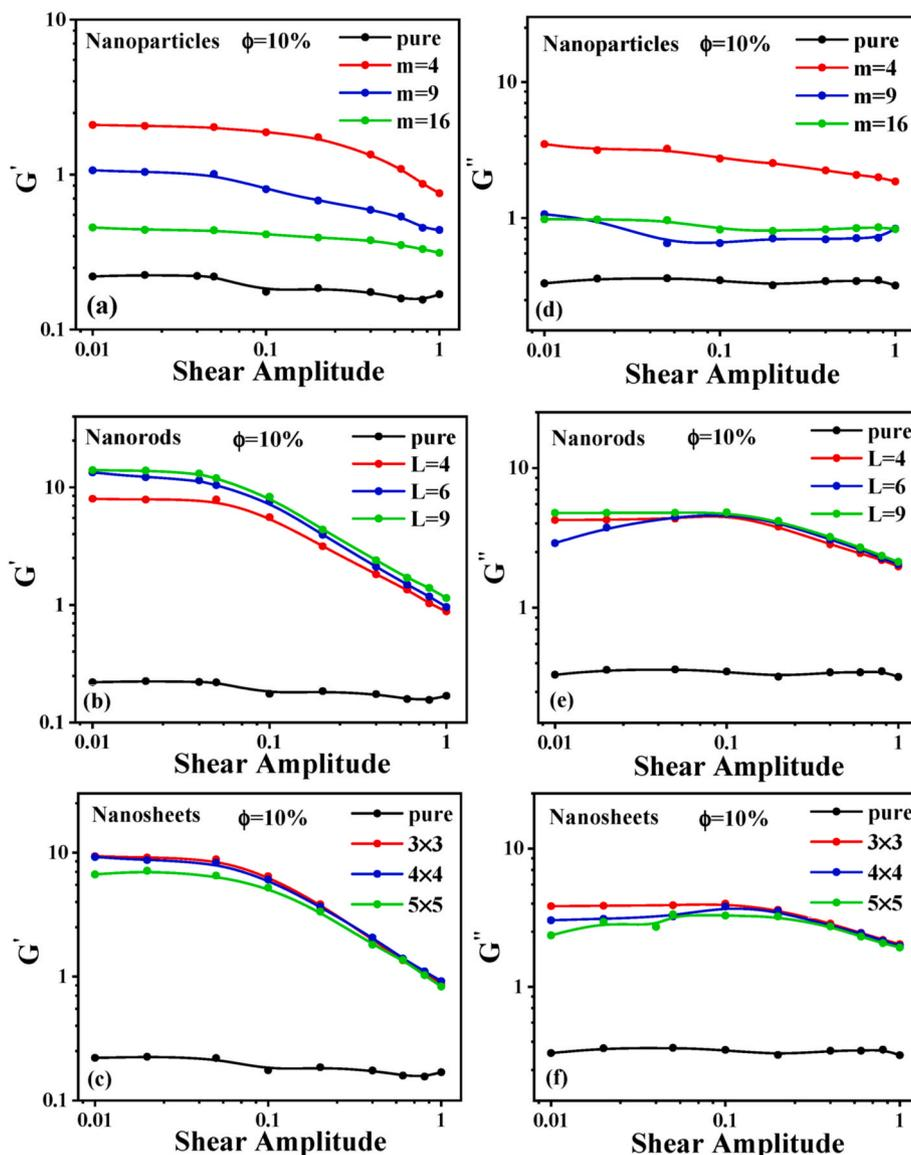
Fig. 3. Variation of energy storage modulus with shear amplitude for PNCs respectively filled with different sizes of (a) nanoparticles, (b) nanorods and (c) nanosheets; variation of loss modulus with shear amplitude for PNCs respectively filled with different sizes of (d) nanoparticles, (e) nanorods and (f) nanosheets.  $\nu = 0.01 \tau^{-1}$ .
