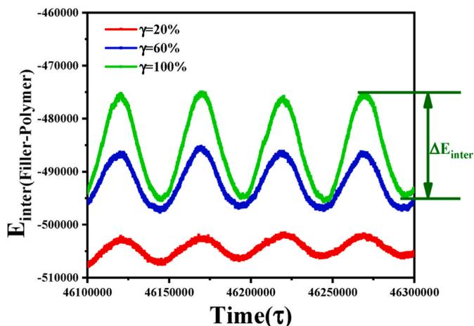
Fig. 9. Schematic diagram of the filler-polymer interaction energy of the system during oscillatory shear.
