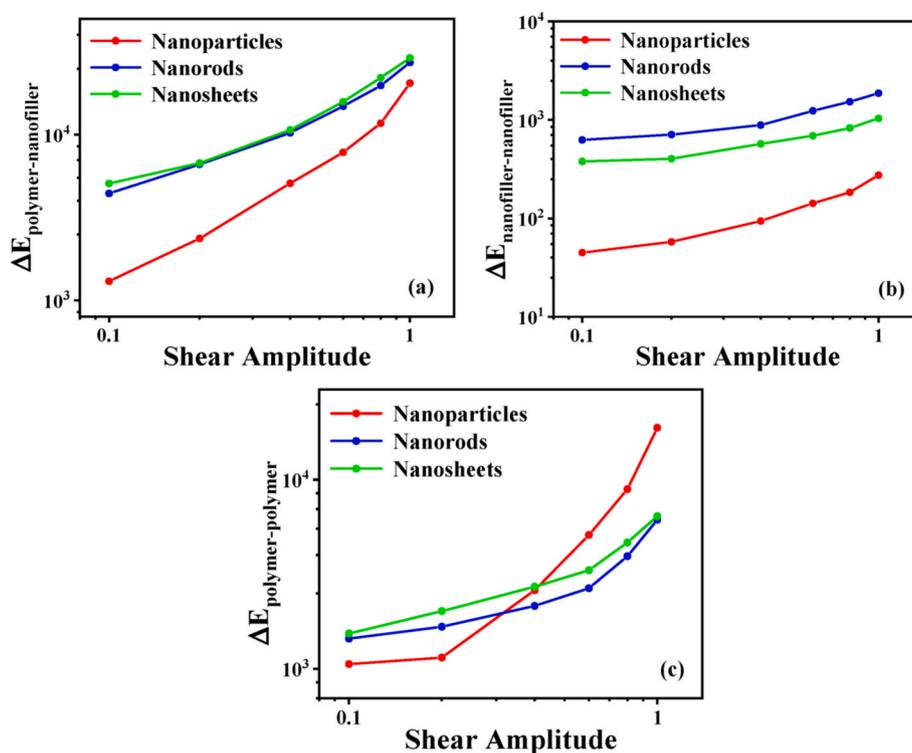
Fig. 10. Variation of (a) polymer-filler (b) filler-filler (c) polymer-polymer interaction energy difference with shear amplitude for PNCs respectively filled with three shape fillers during oscillatory shear,  $\varphi = 20\%$ .
