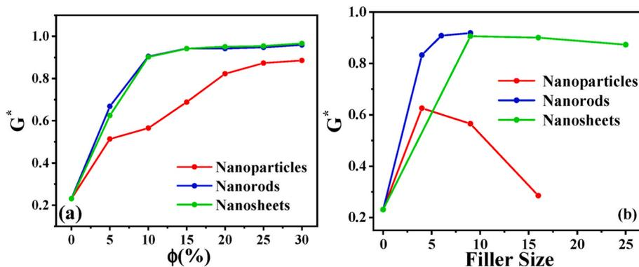
Fig. 4. Quantified Payne effect of PNCs filled with different shapes of fillers as a function of (a) volume fraction and (b) the size of the filler.
