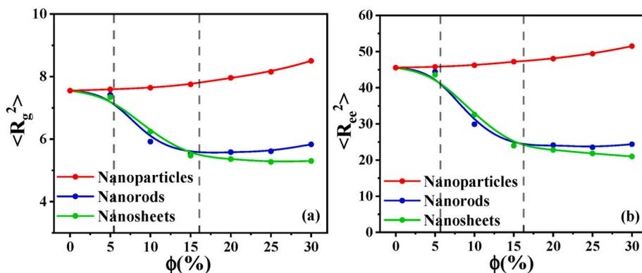
Fig. 7. Variation of (a) mean square radius of gyration ( $\langle R_g^2 \rangle$ ) and (b) mean square end distance ( $\langle R_{ee}^2 \rangle$ ) with filler volume fraction for PNCs respectively filled with different shape fillers.
