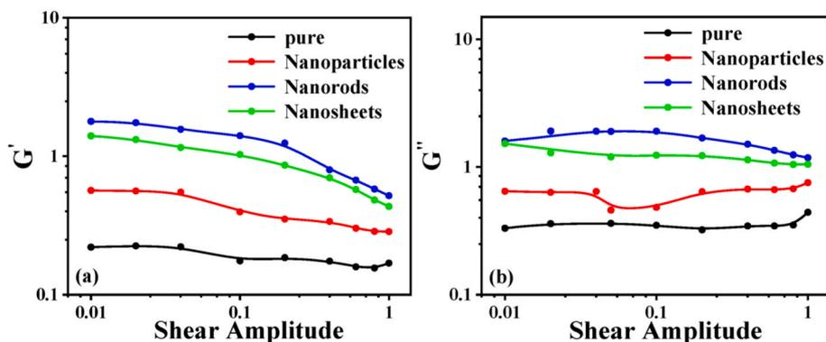
Fig. 2. Plots of (a) energy storage modulus and (b) loss modulus as a function of shear amplitude for PNCs respectively filled with nanoparticles, nanorods and nanosheets, at  $\phi = 5\%$ ,  $\nu = 0.01 \tau^{-1}$ .
