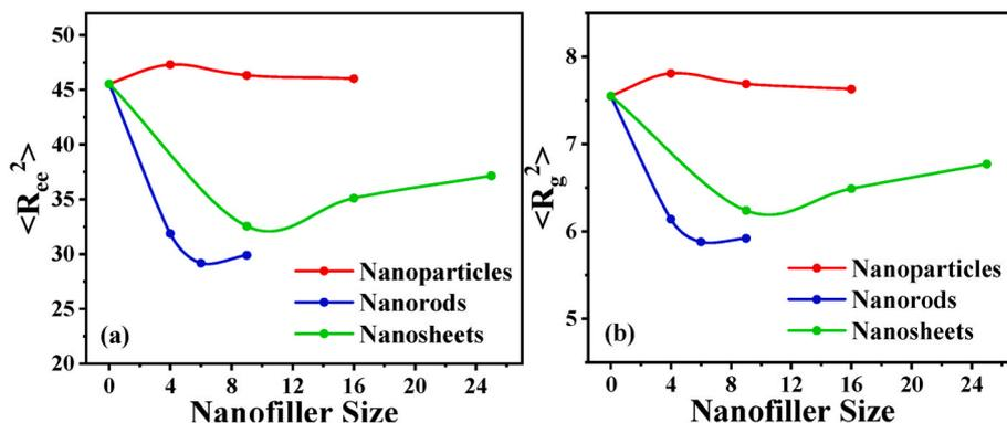
Fig. 8. Variation of (a) mean square end distance ( $\langle R_{ee}^2 \rangle$ ) and (b) mean square radius of gyration ( $\langle R_g^2 \rangle$ ) with filler size for PNCs respectively filled with different shape fillers.
