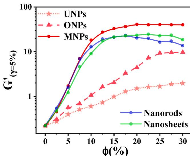
Fig. 11. Variation of energy storage modulus with volume fraction at  $\gamma = 5\%$  for PNCs respectively filled with different interfacial degrees nanoparticles.
