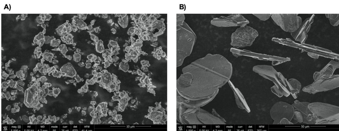
**Figure S1.** SEM images of **A)** alumina trihydrate and **B)** boron nitride fillers.
