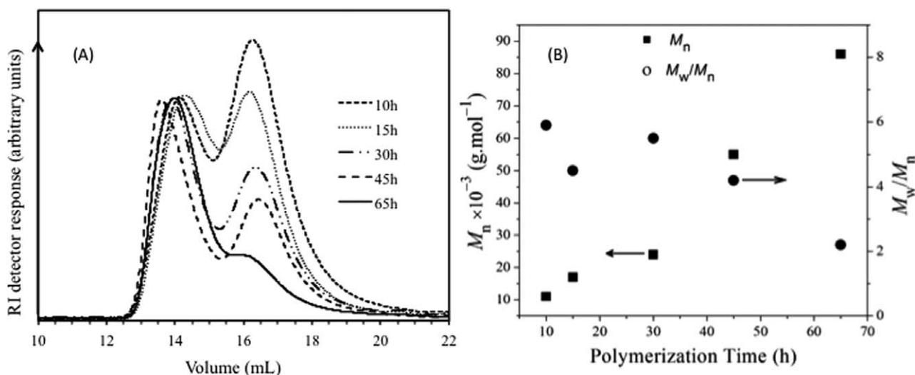
**FIGURE 4** (A)  $M_w$  distribution of polymers obtained with increasing reaction time with similar concentrations of 1, 4-dioxane. (B)  $M_w$  of polymers and their polydispersity with increasing reaction time. Glycidol 12.0 mL; 1,4-dioxane 2.5 mL; 0.125 g of TMP and 95 °C were used for all the polymerizations.
