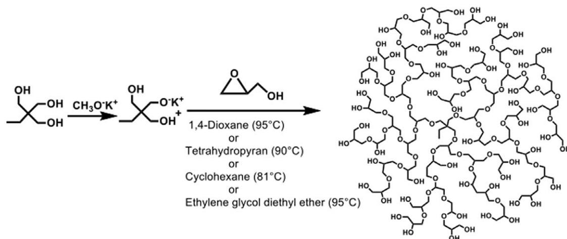
FIGURE 1 Schematic representation of HPG synthesized from TMP initiator in presence of different solvents.
