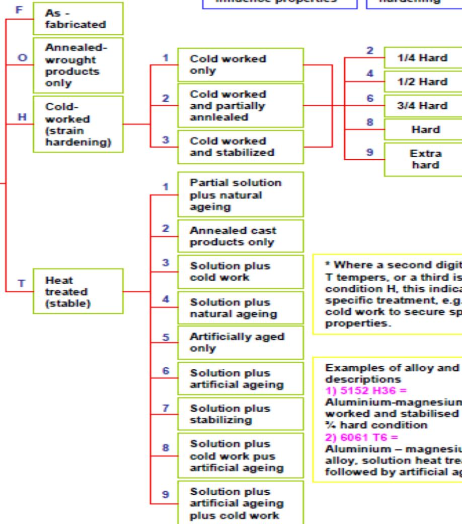
\* Where a second digit is used for T tempers, or a third is used for condition H, this indicates a specific treatment, e.g. amount of cold work to secure specific properties.
