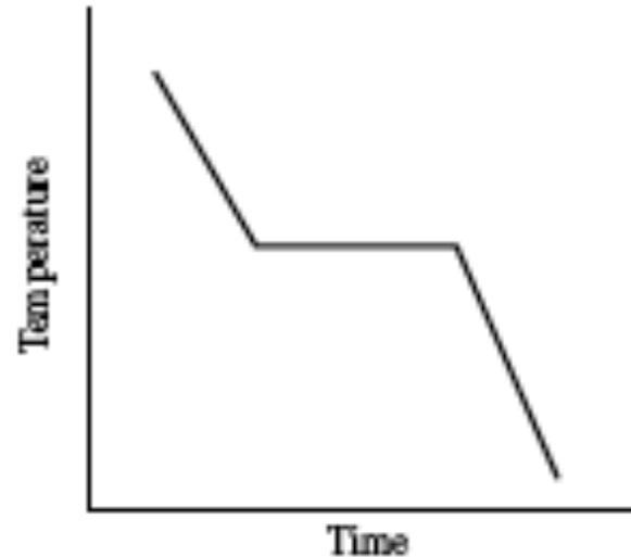
FIGURE 5.11. (a) Schematic representation of the cooling curve for a hypoeutectic alloy revealing the eutectic plateau (see Figure 5.8) and other characteristic landmarks as indicated. (b) Cooling curve for an isomorphous alloy (see Figure 5.3).
