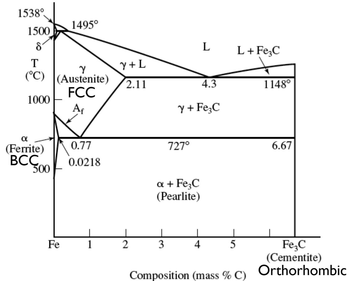
FIGURE 8.1. Portion of the iron-carbon phase diagram. (Actually, this section is known by the name *Fe-Fe<sub>3</sub>C phase diagram*.)  $A_f$  is the highest temperature at which ferrite can form. As before, the mass percent of solute addition is used (formerly called weight percent).
