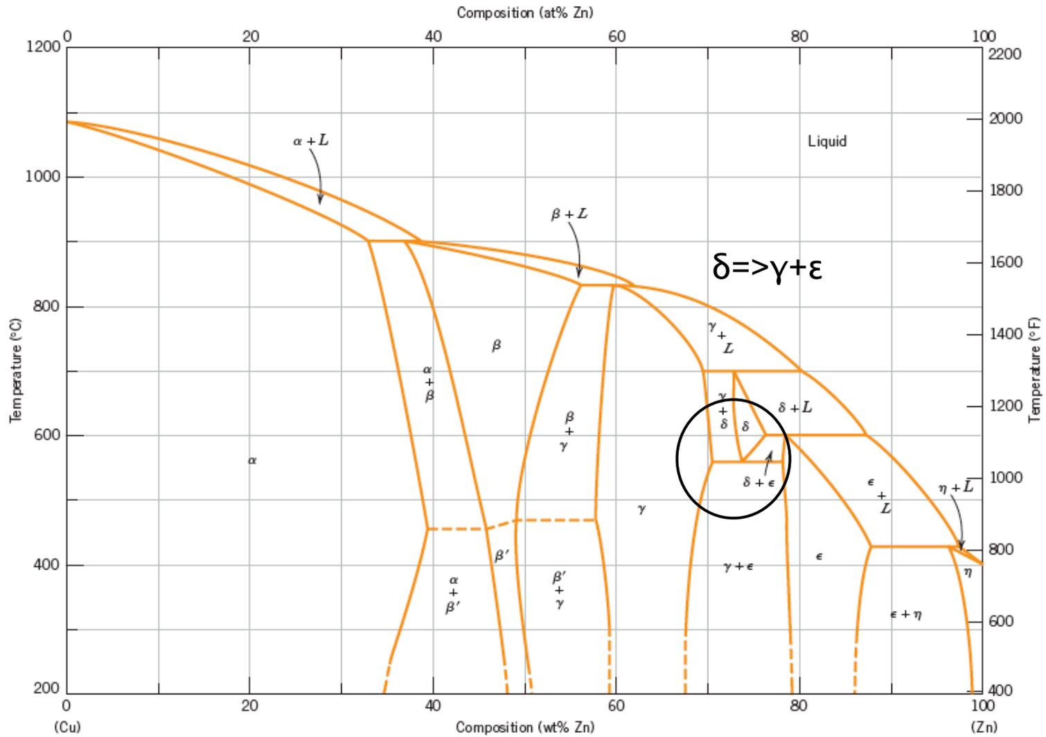
**Figure 9.19** The copper–zinc phase diagram. [Adapted from *Binary Alloy Phase Diagrams*, 2nd edition, Vol. 2, T. B. Massalski (Editor-in-Chief), 1990. Reprinted by permission of ASM International, Materials Park, OH.]
