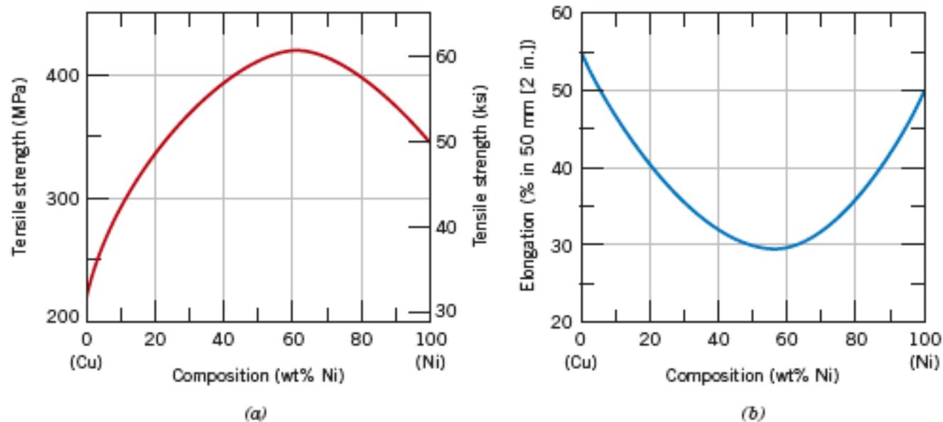
**Figure 9.6** For the copper–nickel system, (a) tensile strength versus composition, and (b) ductility (%EL) versus composition at room temperature. A solid solution exists over all compositions for this system.
