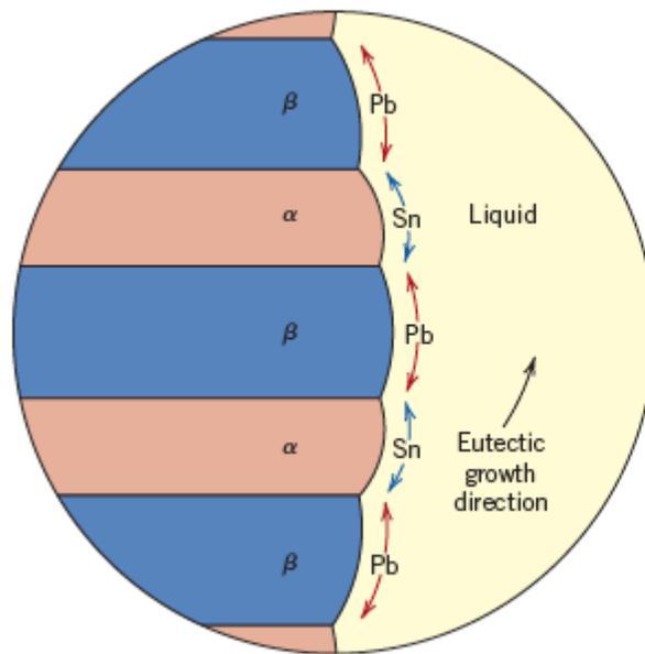
**Figure 9.15** Schematic representation of the formation of the eutectic structure for the lead–tin system. Directions of diffusion of tin and lead atoms are indicated by blue and red arrows, respectively.
