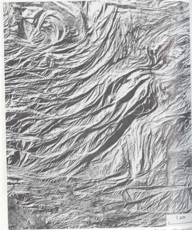
Fig. 4.36. Microstructure of a commercial polyethylene (Rigidex 50) crystallized at 119.8 °C which contains S-shaped, planar and ridged lamellae. Etched surface. (From Bassett, Hodge & Olley, 1979.)
