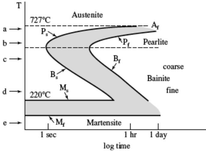
FIGURE 8.4. Schematic representation of a TTT diagram for eutectoid steel. The annealing temperatures (a) through (e) refer to specific cases as described in the text. Note that the hardness scale on the right points downward.
