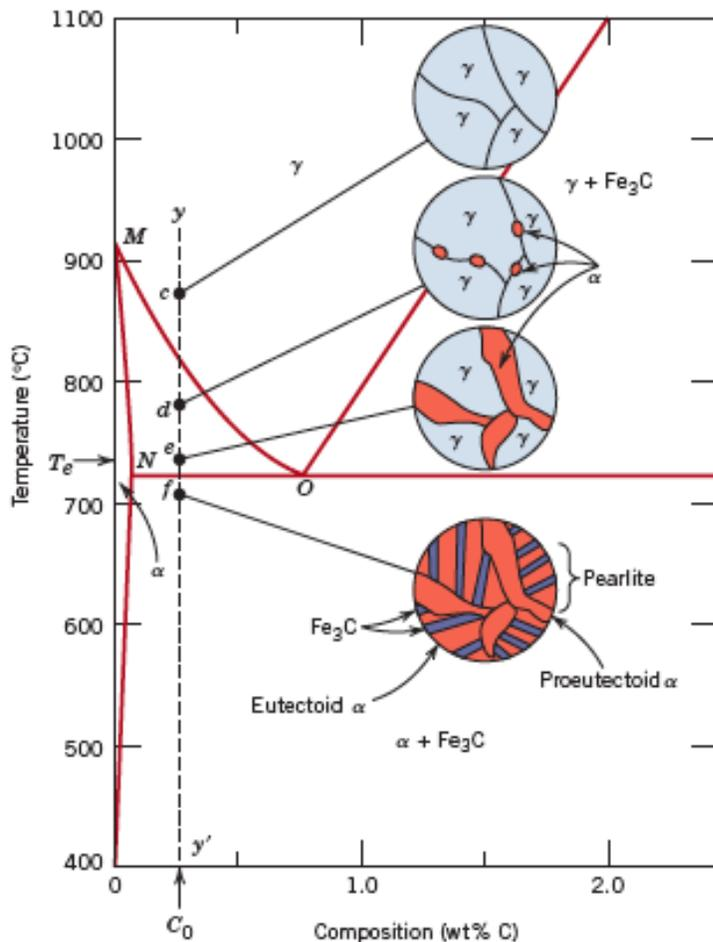
**Figure 9.29** Schematic representations of the microstructures for an iron-carbon alloy of hypoeutectoid composition  $C_0$  (containing less than 0.76 wt% C) as it is cooled from within the austenite phase region to below the eutectoid temperature.
