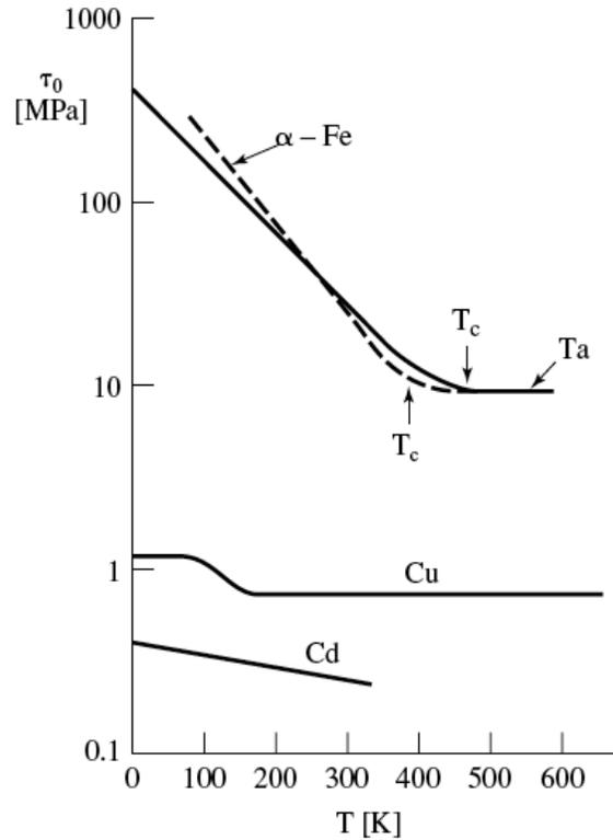
FIGURE 3.23. Schematic representation of the temperature-dependence of the critical resolved shear stress,  $\tau_0$ , for Ta (BCC),  $\alpha$ -Fe (BCC), Cu (FCC), and Cd (HCP) single crystals. Since  $\tau_0$  depends strongly on the crystal orientation, an *average orientation* has been chosen. Specifically, the tensile direction has about the same angle to the [100], [110], and [111] crystal axes. Note the logarithmic scale on the y axis.
