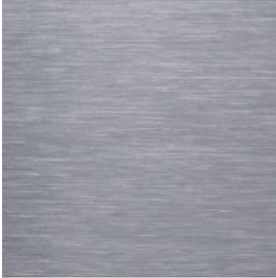
Each stripe is a grain, a single FCC crystal, that has been drawn out. The grains grow from nucleation sites in the melt and prior to drawing they would be randomly shaped grains similar to that seen in the picture of galvanized steel below.
