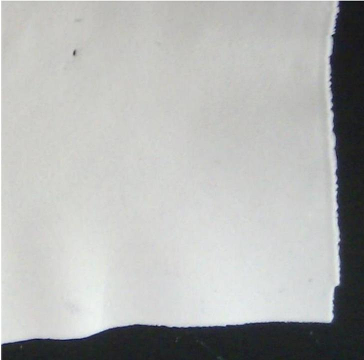
Cellulose based film containing an inorganic filler (1:1 cellulose: filler) cast from an ionic liquid/solvent solution
