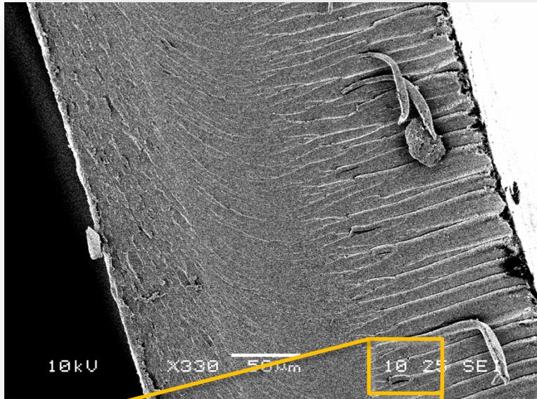
Cellulose film from 15 wt % solution in ionic liquid (cross section)
