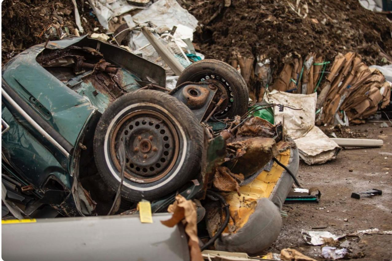
*Seat fibers from a crushed vehicle which will become ASR. Photo credit: Padnos*
