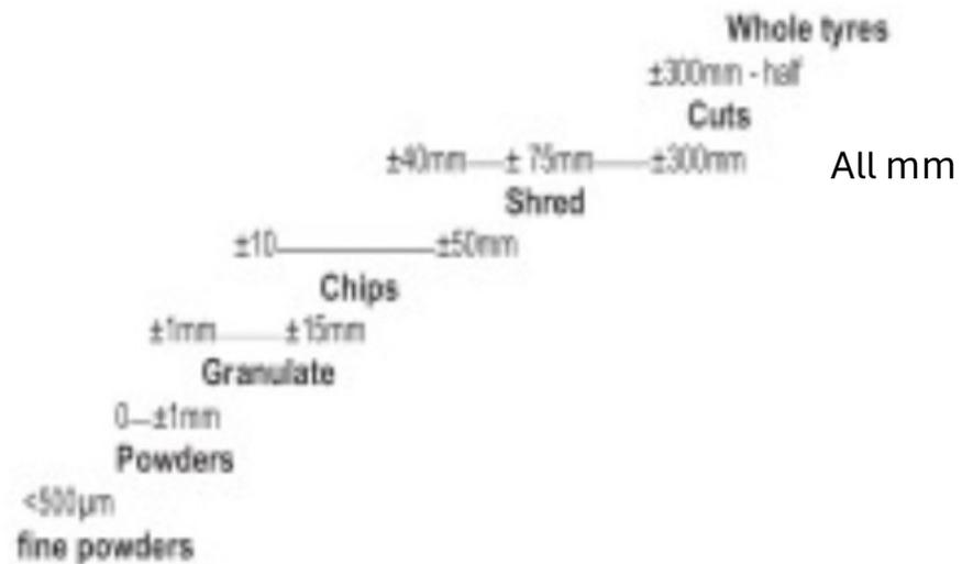
**Figure 4.2** The range of recycled tire materials.
