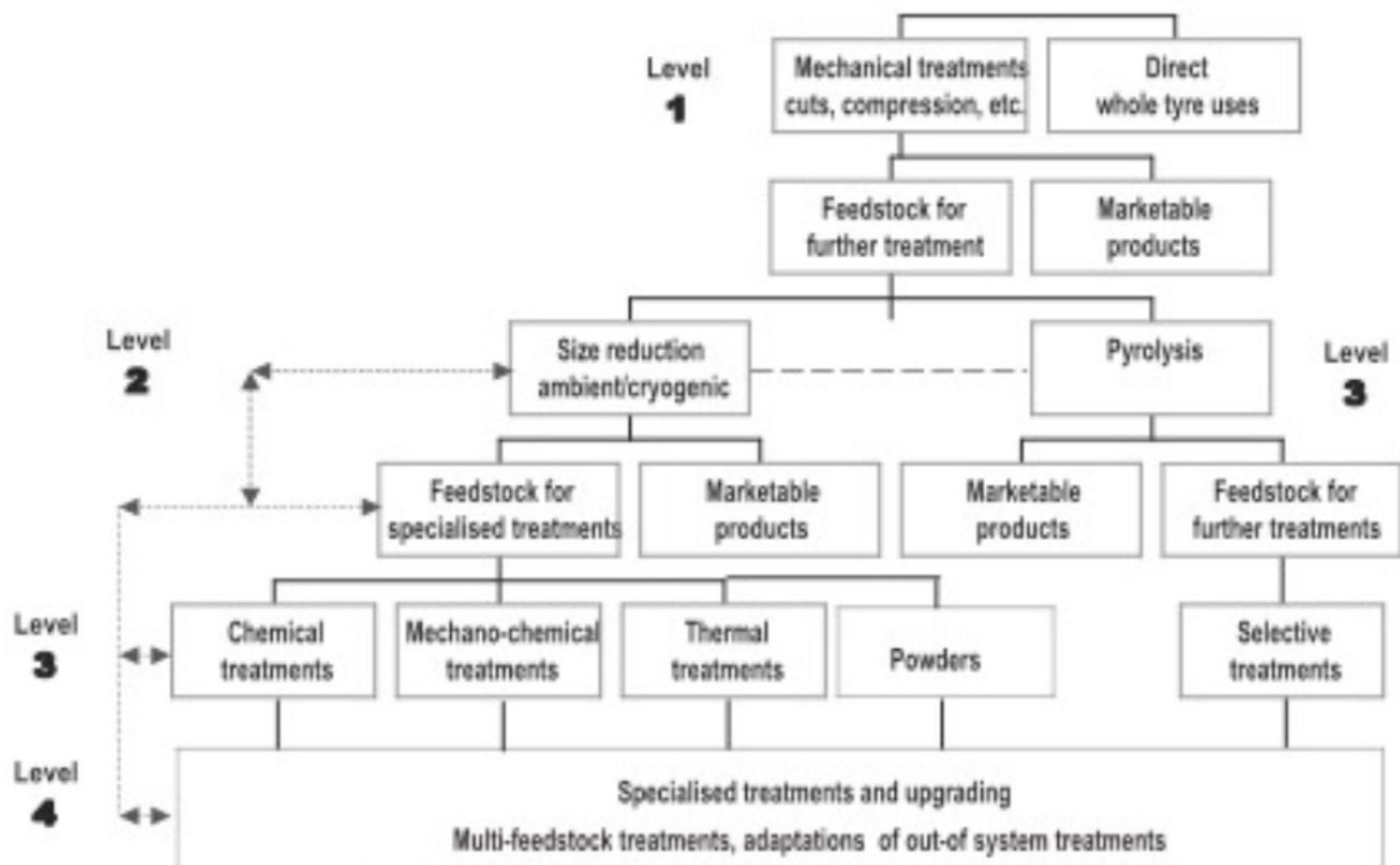
Figure 4.1 Schematic of the four levels of treatment.
