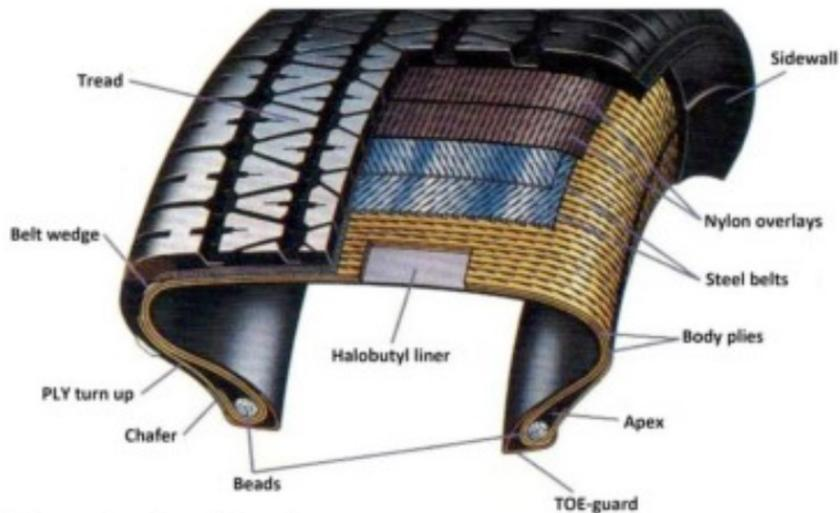
Figure 2.3 Cross-section of a typical car tire.
