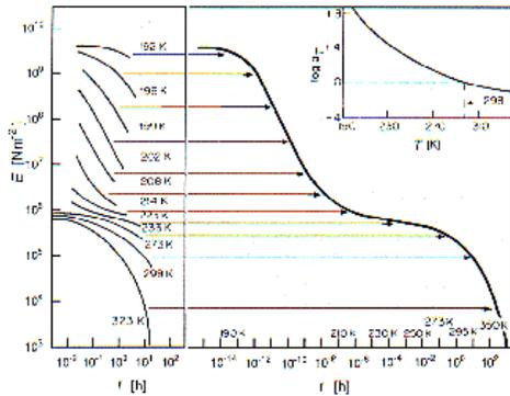
Fig. 5.14. Time dependent tensile modulus of PIB. Measurements at the indicated temperatures (K) and master curve, constructed for a reference temperature  $T = 208$  K (right). The inset displays the applied shifts. Data from Cassill and Tobolsky [5.4].
