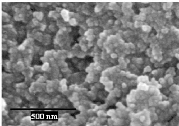
*Figure 2. Representative SEM of silica-C<sub>60</sub> hybrid synthesized by scheme 2 (reproduced from ref. 10).*
