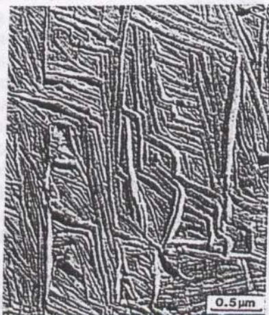
Fig. 31. Ridged crystals in linear polyethylene (photograph supplied by D.C. Bassett; first published in [3]).
