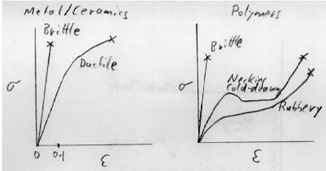
2) a) In metals the morphological basis for yielding (ductile curve above) is generally given as edge dislocations.
