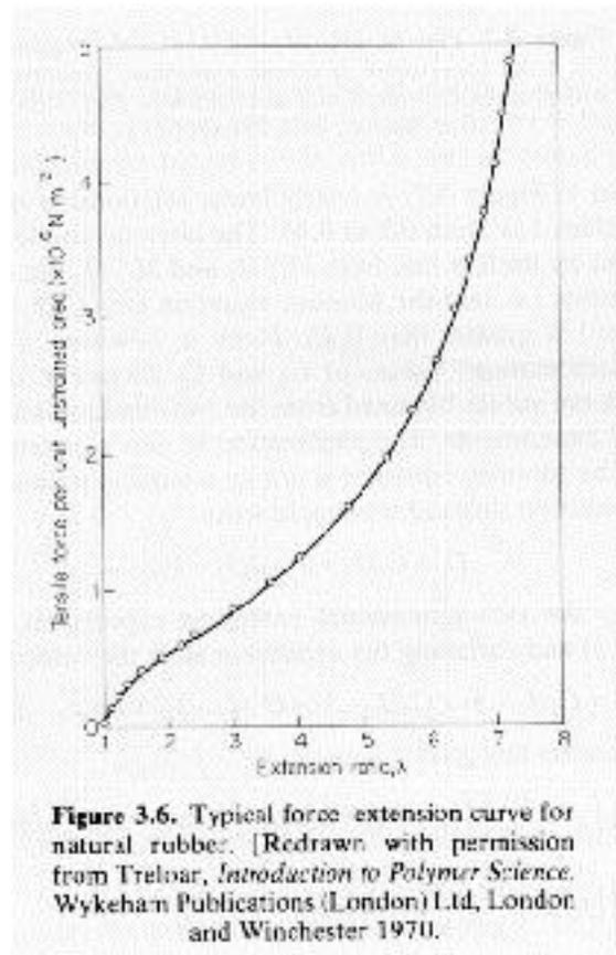
**Figure 3.6.** Typical force-extension curve for natural rubber. [Redrawn with permission from Treloar, *Introduction to Polymer Science*. Wykeham Publications (London) Ltd, London and Winchester 1970.
