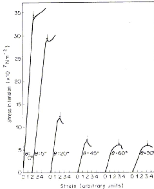
Figure 11.28. Stress-strain curves for various angles  $\theta$  between the tensile axis and the initial draw direction for tensile tests on drawn polyethylene terephthalate sheets. The yield points are marked by arrows. [Redrawn with permission <http://www.eng.uc.edu/~gbeaucag/Classes/Characterization/>]
