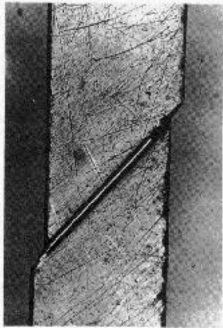
Figure 11.26. Photograph of a deformation band in an oriented sheet of polyethylene terephthalate.
