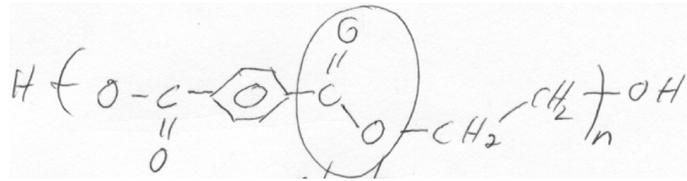
Glyptal has di ortho carboxylic substituted aromatic group and PET has di para substituted aromatic group. This makes PET more flexible than glyptal. Also, the trifunctionality of glycerin versus the difunctionality of ethylene glycol leads to a network structure that is more rigid compared to PET.
