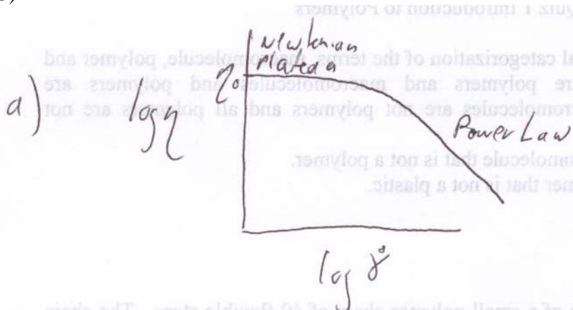
b) At high rates of strain the viscosity drops so it becomes easier to process. This is called shear thinning.
