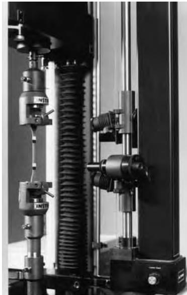
Figure 3-12. Optical Extensometer
