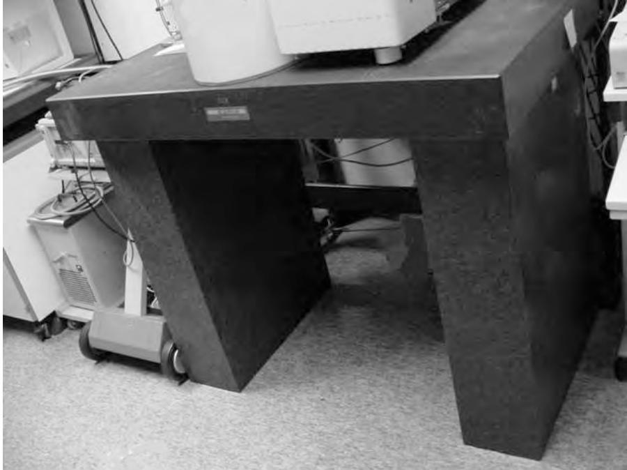
The above picture shows a suitable stone bench on which the DMA/SDTA861<sup>e</sup> can be installed.
