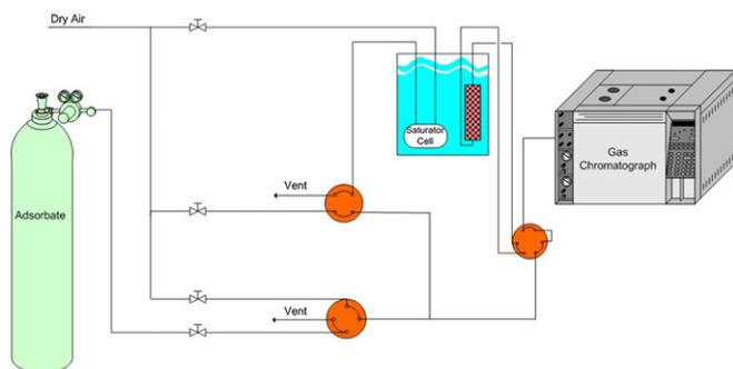
**Fig. 2.** Rapid nanoporous adsorbent breakthrough testing apparatus.
