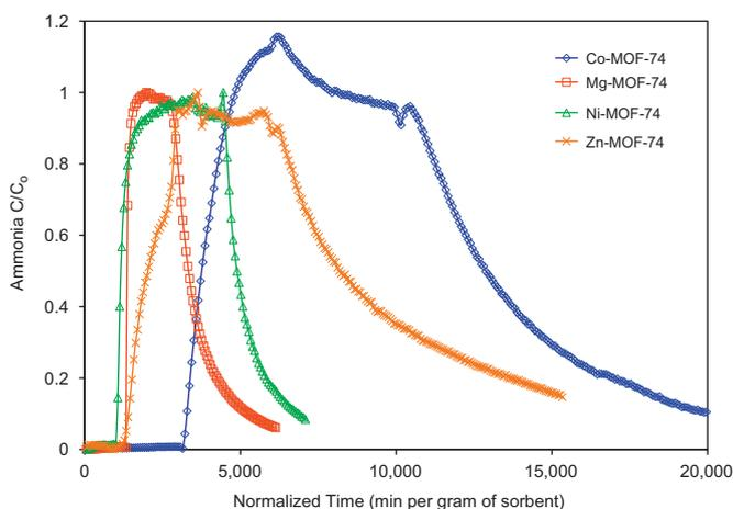
Fig. 8. Ammonia breakthrough curves under humid (RH=80%) conditions.
